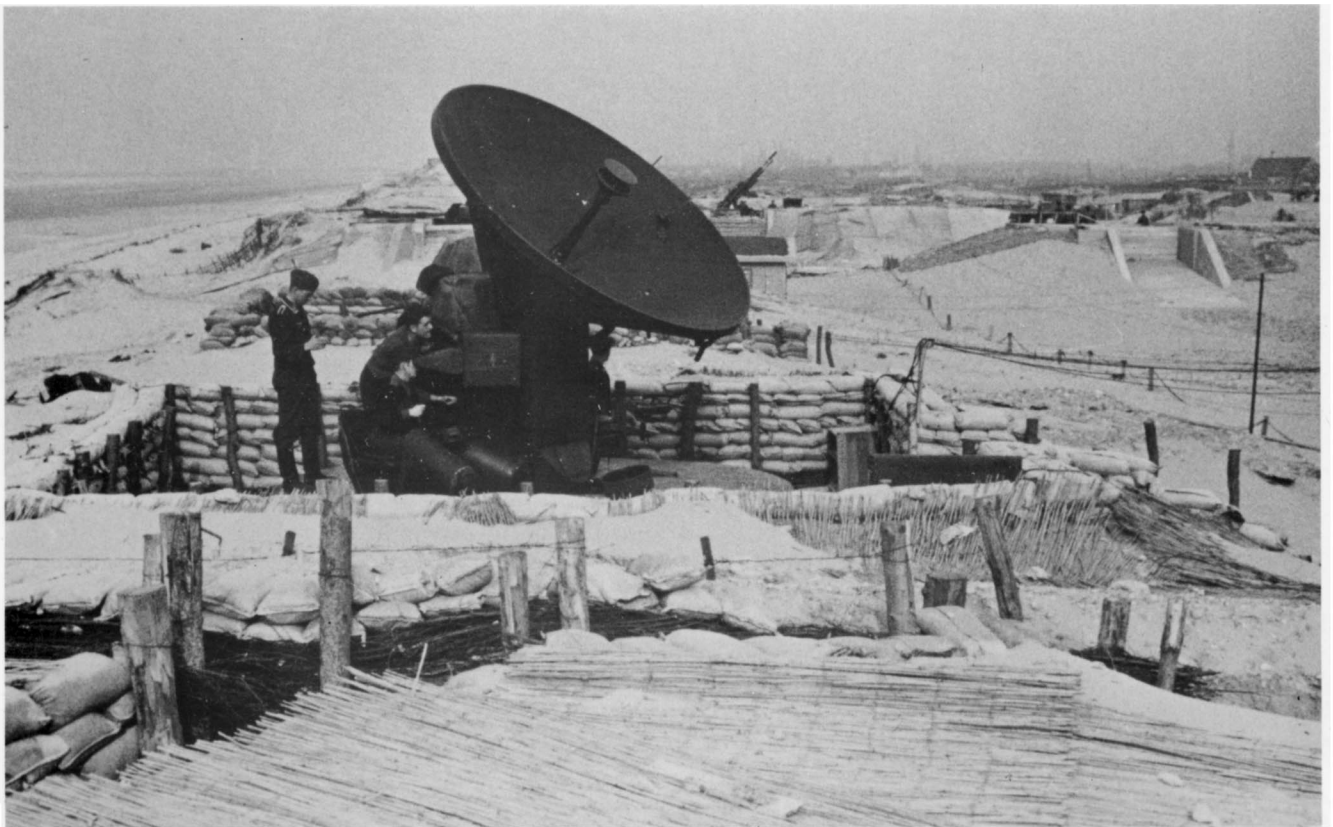
Above: This FuMG 39 T D has been set up here along France's Atlantic coast in a well-fortified 88 mm gun emplacement.
