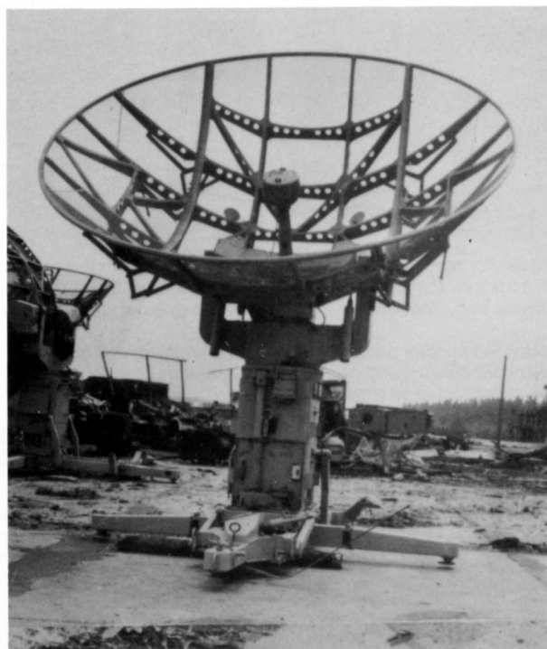
Two photos of the FuMG 68 Ansbach. It consisted of a Drehstand 68 pivot stand with the remotely controlled 4.5 m reflector dish and the Bedienungswagen 68 operations van (below). The perforated parabolic dish rested with its pivot shaft on a cross base.
