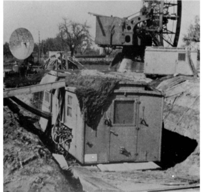
Above: The controls for both radars and the instrumentation were housed in the Bedienungswagen 74/76 Bayern operations van.
