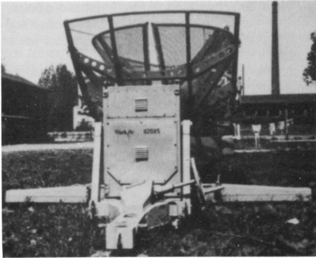
In order to be transported on the Sd.Ah. 204 two segments of the overly wide reflector had to be detached and folded in toward the center of the dish. The pivot shaft was lowered to its horizontal transport position and raised to its operating position by hand. See photos.
