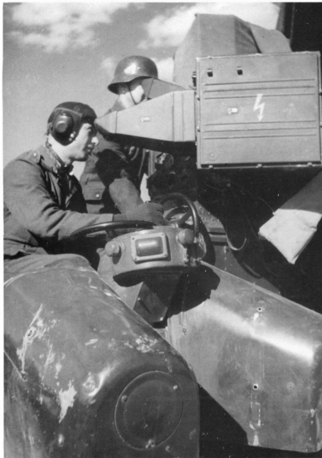
Above left: Here we see the B2 in the foreground, sitting in the control seat where he's moving the system on its lateral axis. He is looking into the range and bearing indicator in front of him. Behind him stands the B3 at the elevation monitoring scope and is operating the elevation crank on the radar housing.
