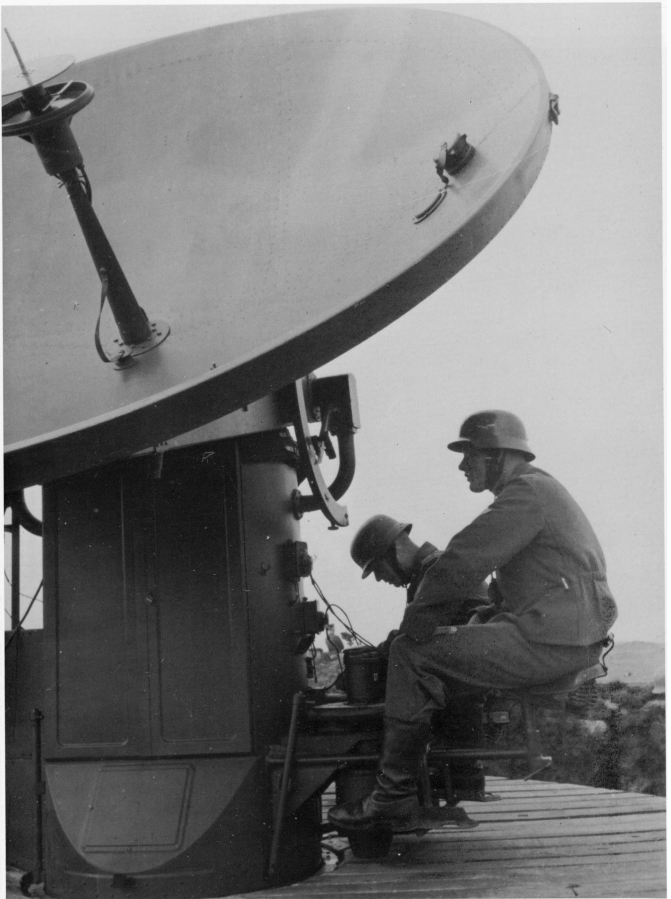
The Würzburg C system had a rotating antenna and a new ANG 62 scope. Located on the inner lip of the reflector dish is one of the IFF dipoles with its protective cap on. Just opposite this, on the dish's outer lip, is one of the two snap locks which hold the two dish halves together. These are two of the crew members; the B6 sits in front of the elevation quadrant and the B5 at the azimuth scale. Both were to pass their respective data on to designated command and control centers or searchlight units by voice radio in the event that the Übertragungsgerät 37 was not operating.
