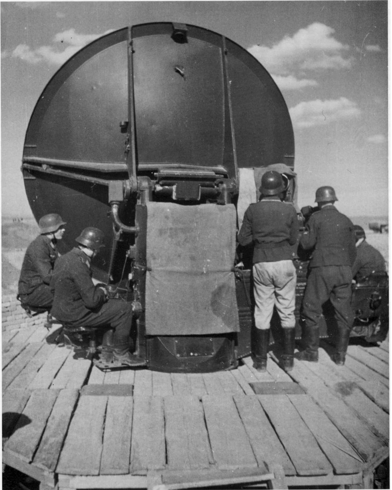
This is an FuMG 39 T D2 or D3 with its wooden traverse plate. The crew, seen in position, are as follows (from left to right): The B6 seated at the elevation quadrant passed the altitude information by voice radio to a command and control center or to an associated searchlight unit. Next to him, the B5 sitting at the bearing indicator instrumentation passed this information on by radio as needed. The B1 stands at the rangefinder, a cathode ray tube (CRT). Next to him is the B3 standing at the height tracking scope, while the B2 sits in the control seat, where he controls the elevation angle and bearing of the system. If the Übertragungsgerät 37 were not operating, the B4 would stand next to the B1 at the rangefinder to pass on ranging information via radio.
